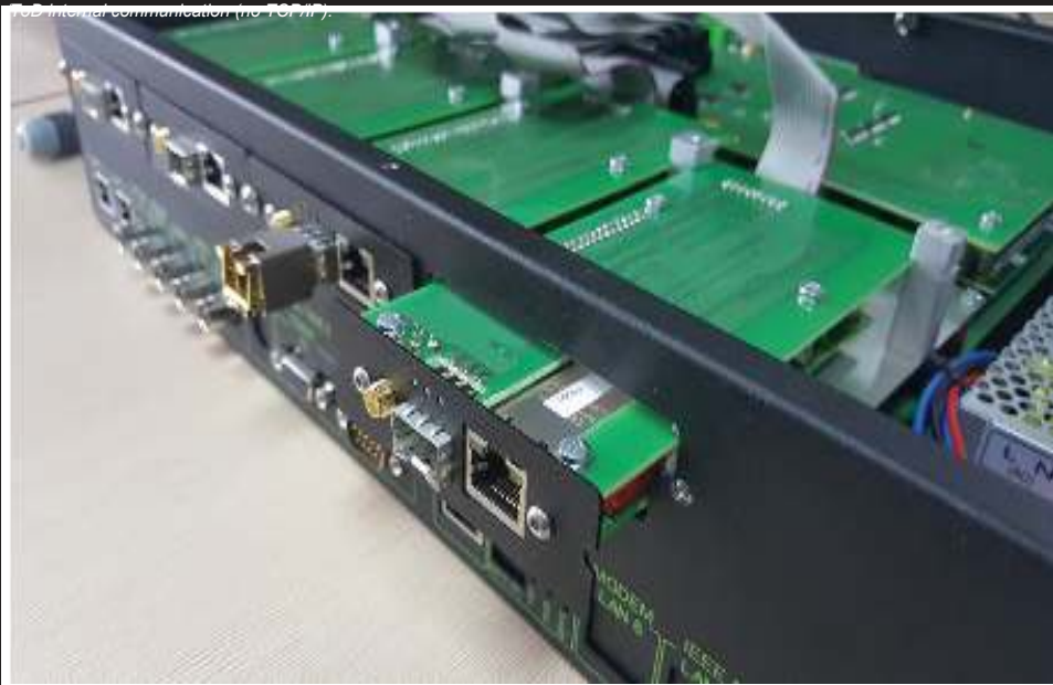
4x NIC (EXPANDER 1-4) are 100% isolated from each other. There is analog communication between NIC and NTS-5000 (no TCP/IP)
