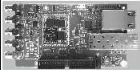
All NIC cards are 100% isolated from each other using analog PPS & internal communication (no TCP/IP)
